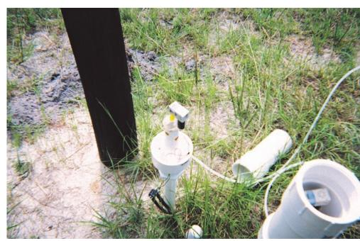
A one inch diameter monitoring well was installed in each lysimeter to facilitate sampling of the accumulated rainwater. Periodically, as the lysimeters fill, the water is collected and sent to the laboratory for analysis.
